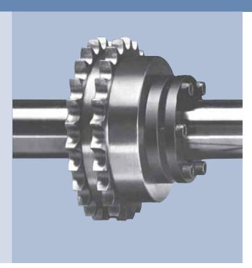
The ETP shaft bushing is a high-quality clamping element, which mounts components such as sprockets, toothed wheels, levers and other machine parts fast, easily and permanently onto shafts. Grooves, tapers and inside threads are no longer necessary.
