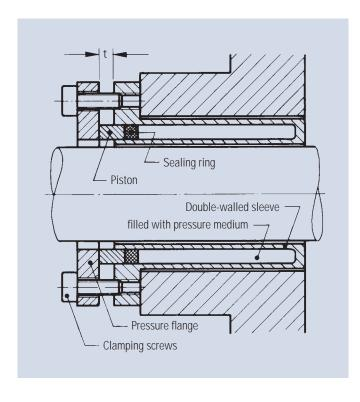
The ETP bushing consists of five parts: double-walled sleeve filled with pressure medium, sealing ring, piston, pressure flange and clamping screws (3, 4, 6 or 8 screws).
