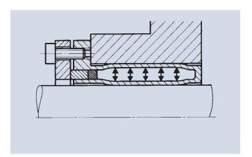
Fine adjustments are possible. Adjusting the transmission elements is never a problem. The bushings are subsequently radially and axially adjustable to change positions without difficulty and backlash-free.
